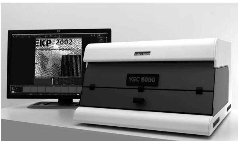
Figure 10.1 The video spectral comparator (VSC 8000) made by Foster and Freeman Ltd. (Evesham, Worcestershire, UK). This instrument enables examination of documents in infrared and ultraviolet luminescent and absorption conditions to be carried out. A document placed inside the cabinet is viewed on the monitor screen. A wide variety of lighting conditions are available for the observation of the document as well as image processing facilities.
