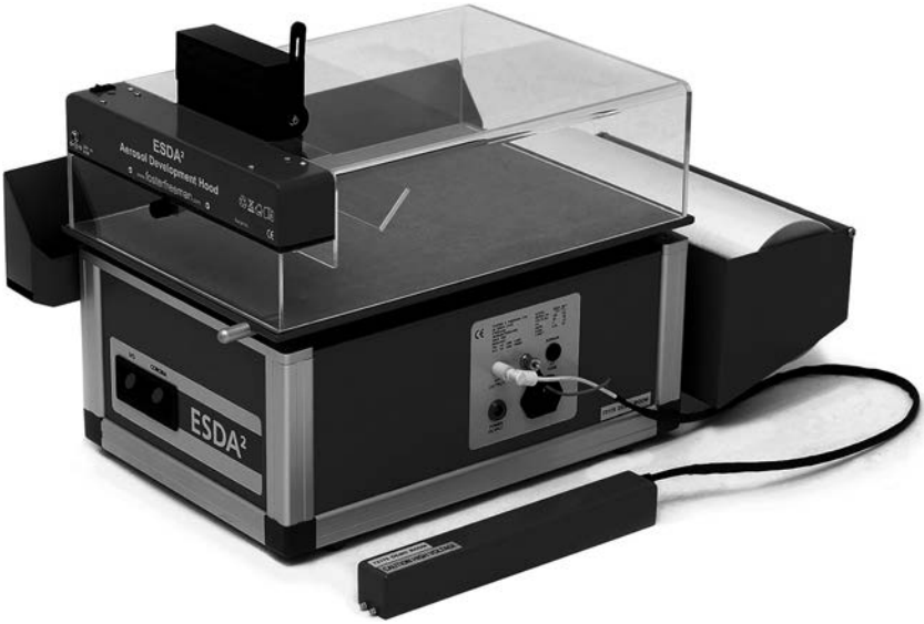
Figure 9.1 The electrostatic detection apparatus (ESDA) made by Foster and Freeman Ltd.
