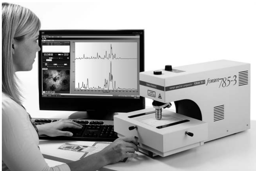
Figure 10.2 The Forum 3 made by Foster and Freeman Ltd. (Evesham, Worcestershire, UK). This instrument enables the capture of Raman spectra, a form of vibrational spectroscopy that can assist in distinguishing between different inks.
