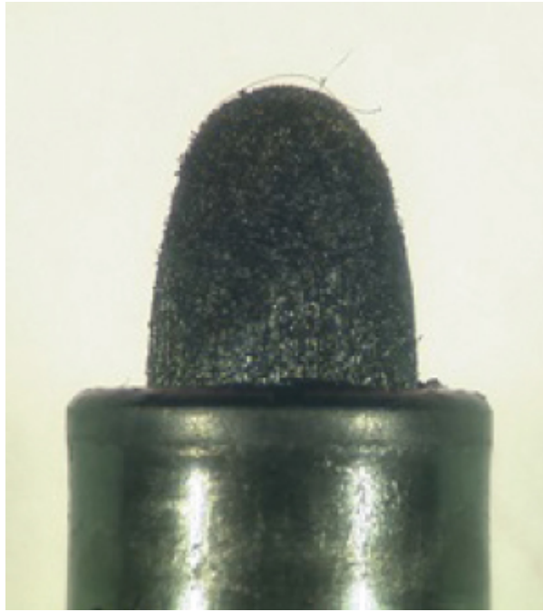
Figure 2.7 A felt tip pen nib (x8 approx.).
