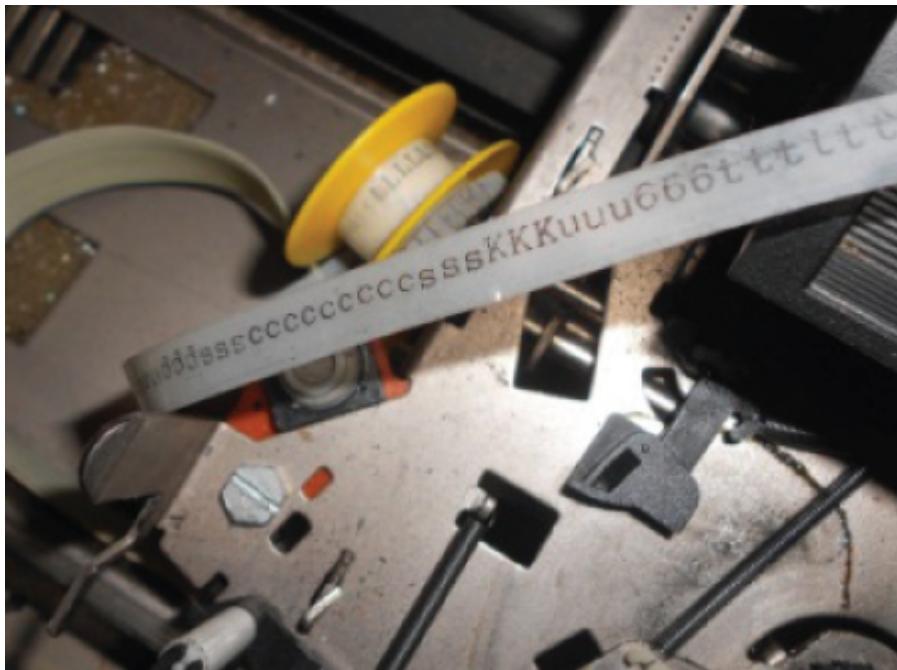
Figure 4.12 A lift off correction ribbon with removed characters present.
