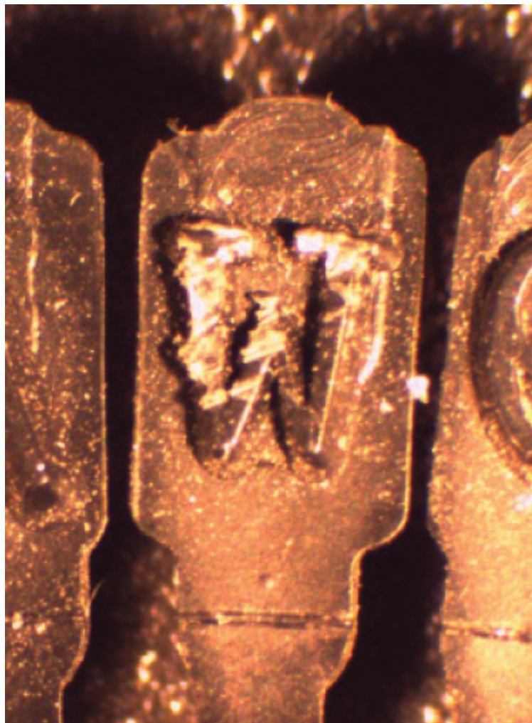
Figure 4.10 Close up of a severely damaged letter w on a printwheel (x10 approx.).
