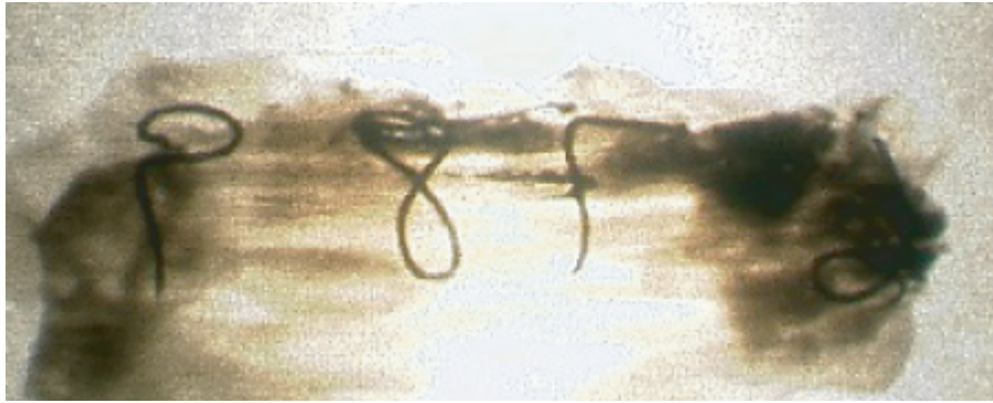
Figure 8.6 An entry covered with correction fluid viewed from behind the document illuminated with transmitted light.
