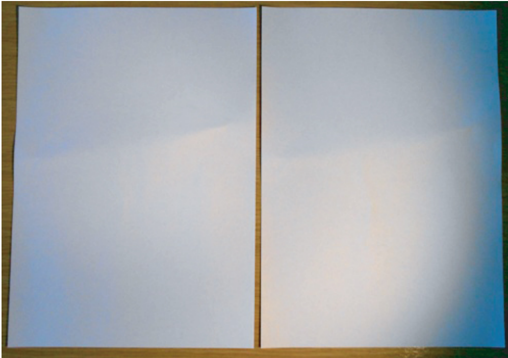
Figure 8.2 Two pieces of paper with similar crease patterns viewed under oblique light.
