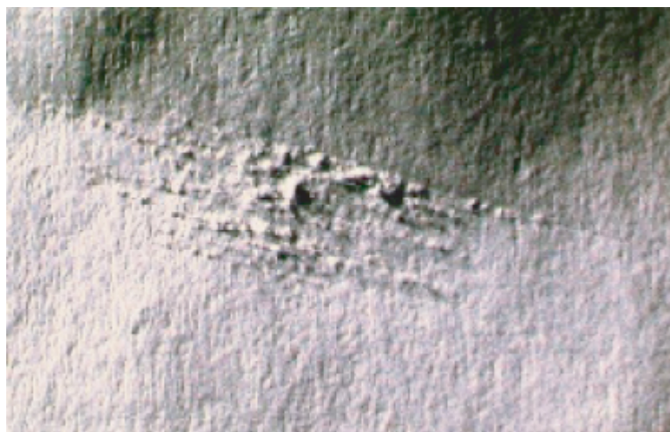
Figure 8.4 Oblique light view of an abraded document close up (x3 approx.).
