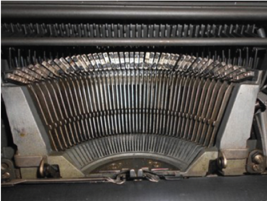
Figure 4.1 The arrangement of typebars.
