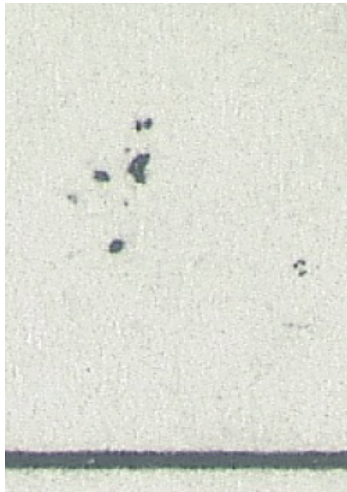
Figure 4.15 Close up of a group of drum defects (x15 approx.).
