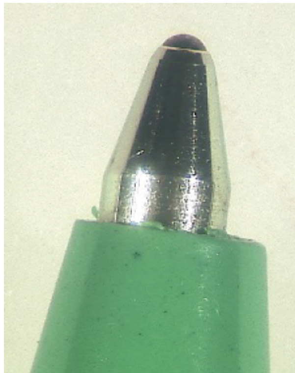
Figure 2.5 The tip of a ballpoint pen (x8 approx.).
