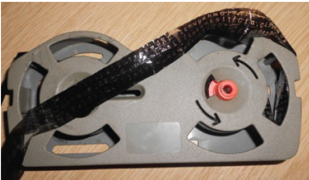
Figure 4.11 A carbon film ribbon showing readable text after use.
