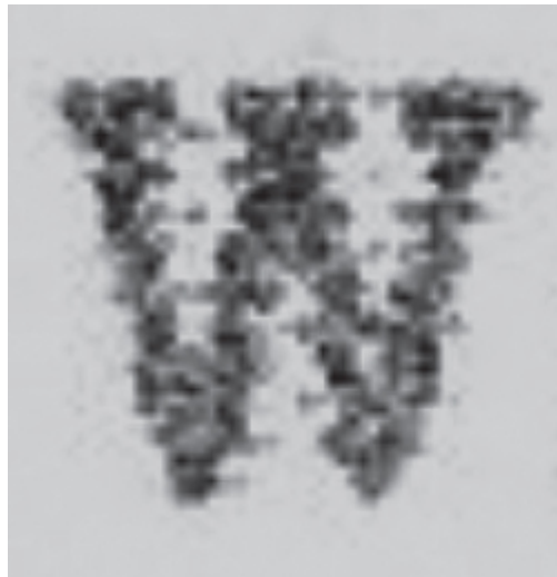
Figure 4.5 Close up of letter w showing the weave pattern from the fabric ribbon (x15 approx.).
