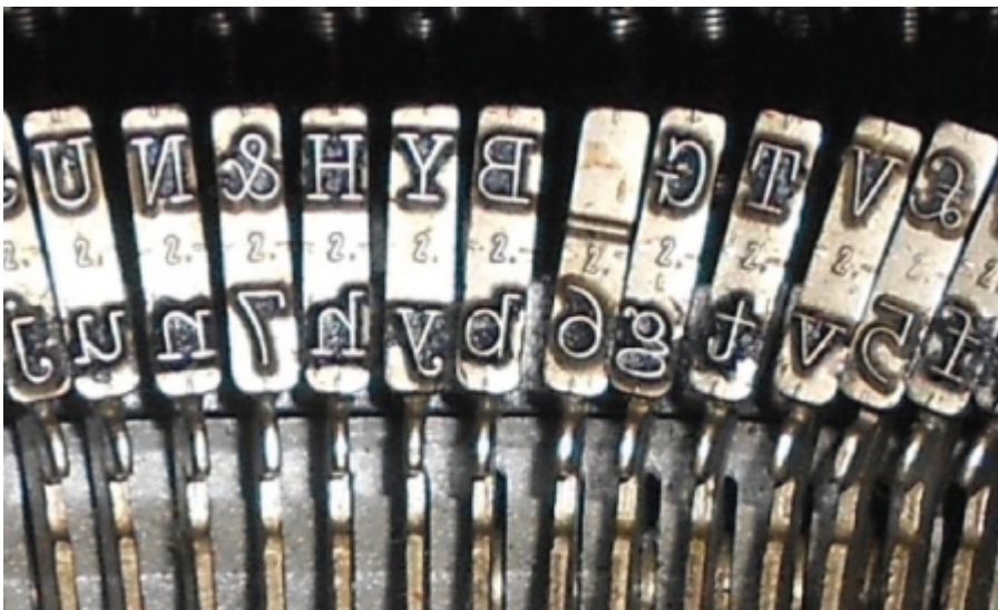
Figure 4.2 Two characters are present at the end of each typebar with the upper one accessed by using the shift mechanism (x3 approx.).
