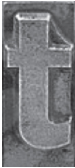
Figure 5.3 A letterpress printing surface (x25 approx.).
