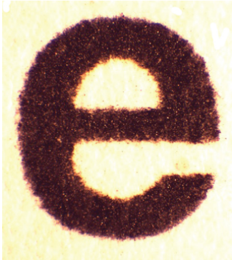
Figure 4.14 Letter e printed with a laser printer showing the molten appearance of raised toner on a paper surface (x30 approx.).
