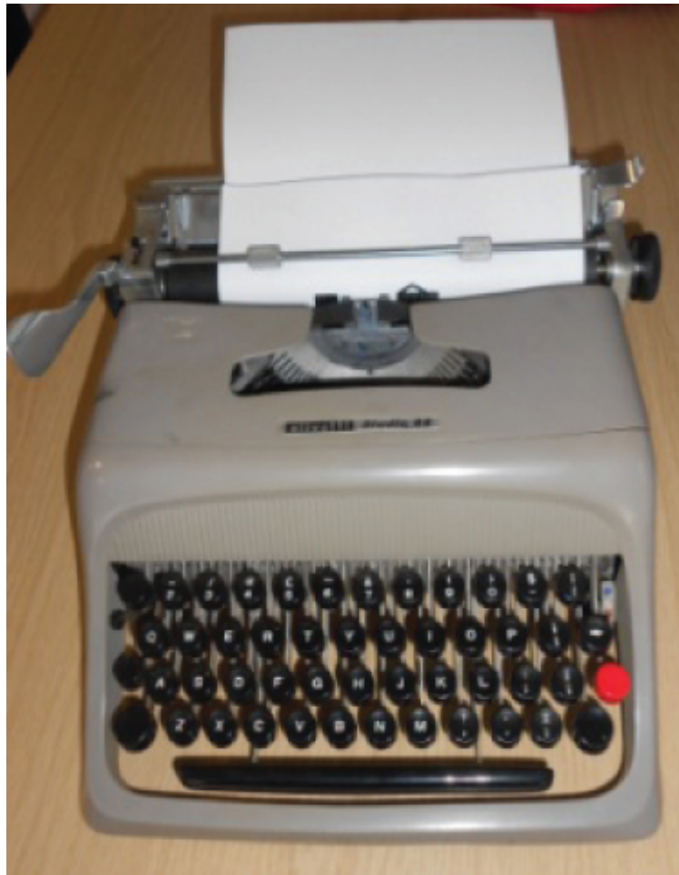
Figure 4.4. Paper inserted round a typewriter platen.
