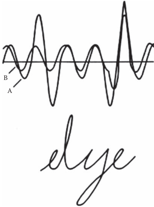
Figure 3.3 Effect of changing the stiffness of a two-dimensional spring model of robotic handwriting. Vertical (A) and horizontal (B) velocity components generated by the mass spring model and the resultant writing trajectory. (From Hollerbach, J. M. 1981. Biological Cybernetics 39:139–156. With permission.)
