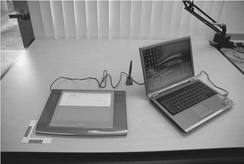
Figure 7.4 Wacom Intuos 3 digitizer tablet and laptop computer. MovAlyzeR software installed on the computer is used to acquire and process signature samples.
